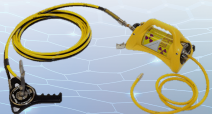
Figure 3: Gamma radiography equipment (GED) - DELTA Sentinel 880 with Ir-192 source.
