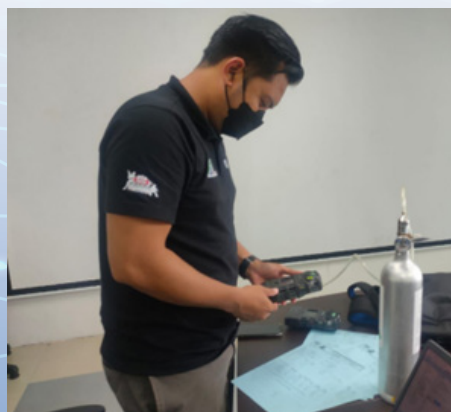
Figure 16 : Site Calibration Portable Gas Detector at NIOSH Regional Office
