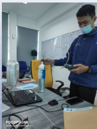
Figure 16 : Site Calibration Portable Gas Detector at NIOSH Regional Office
