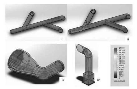
Figure 6: Air flow streamline in (i) inlet a (ii) inlet b (iii) inlet c and iv) outlet for type 2
