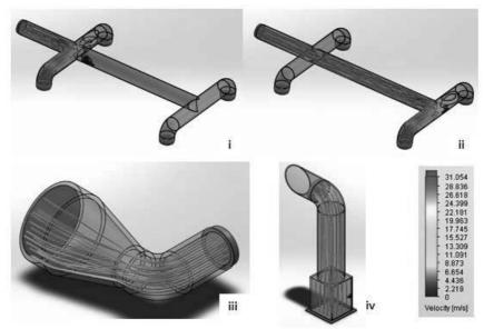
Figure 5: Air flow streamline in (i) inlet a (ii) inlet b (iii) inlet c and iv) outlet for type 1
