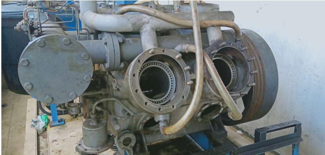
**Figure 13.4.** Abandon compressor pump before the complete maintenance at the factory causing the residual ammonia to release at the opening. (Source: DOSH 2020)
