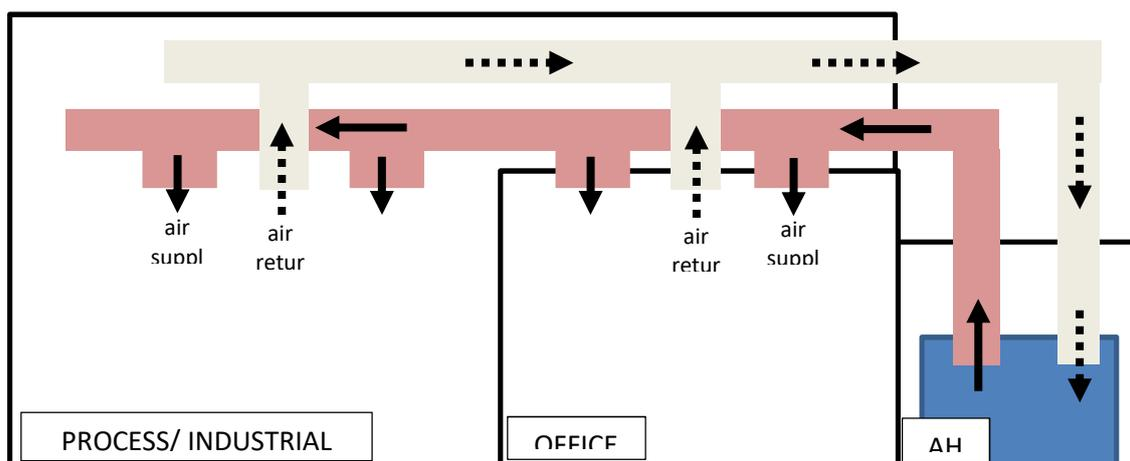
*Figure 16.1. Possible Mistake for MVAC Air Distribution for Industrial Office*
