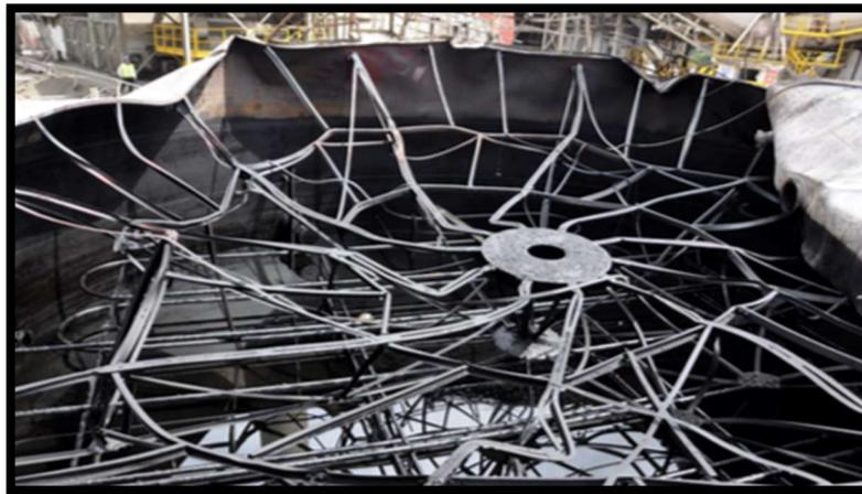
Figure 10.3. The wall structure of the storage tank bent inward and the heating coil inside the tank
