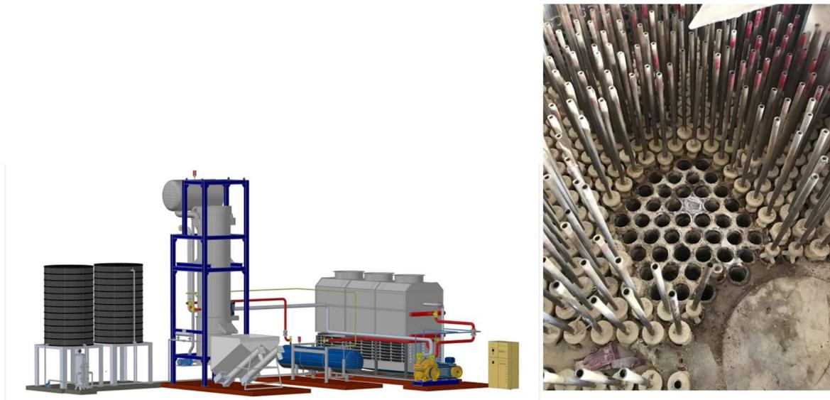
**Figure 13.2.** Typical ice making refrigeration system (left) and the plugged tube that cause the accident (right).
