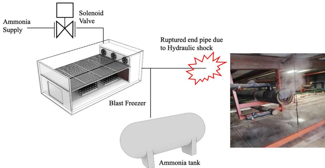
**Figure 13.1.** The simple diagram of pipeline connection of the related components involved with the accident and the visible ammonia at cloud at the end pipe after the accident even though several attempts have been conducted to shut all the supply valves (Source: DOSH 2019)
