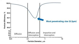
To boost performance in this critical size range, many masks use fibres that have a static charge<sup>[6]</sup>. Disinfecting mask using alcohol removes this charge. **Bottom Line is alcohol deactivates viruses, but it significantly reduces filtration effectiveness.**
