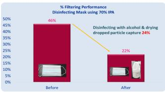
The DML lab tested particles size around 0.3 microns using TSI Model 8130 Automated Filter Tester to measure filter aerosol penetration.
